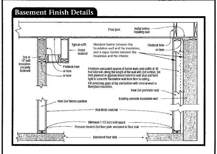
This prescriptive example assumes the prior application of dampproofing or water-proofing on the exterior of the concrete foundation
