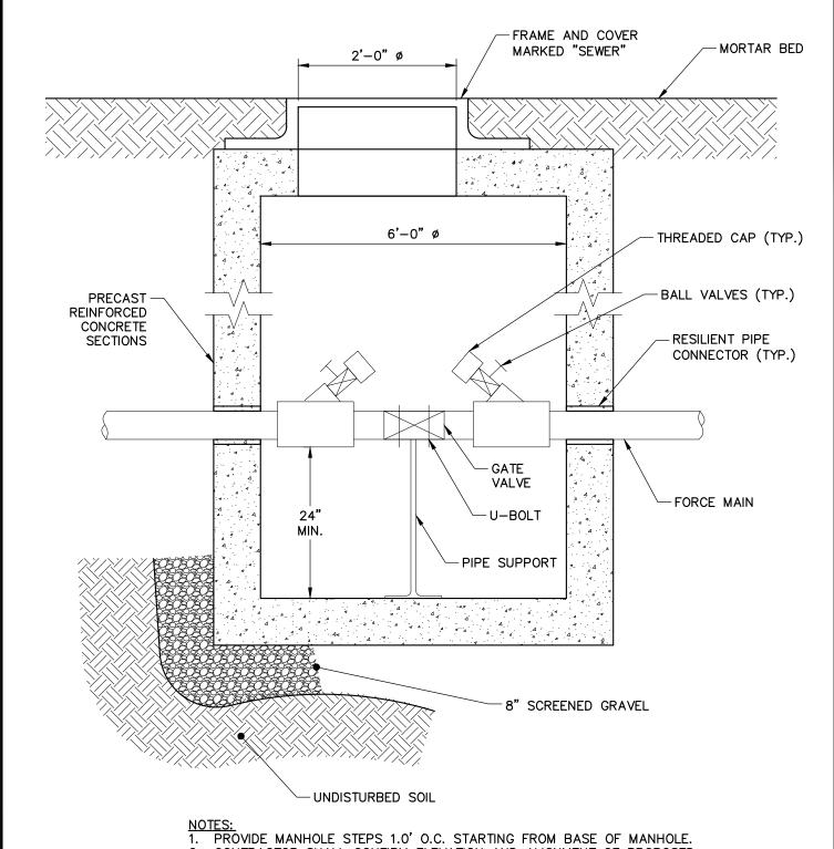
2. CONTRACTOR SHALL CONFIRM ELEVATION AND ALIGNMENT OF PROPOSED FORCE MAIN AND GROUND SURFACE AT EACH MANHOLE PRIOR TO ORDERING SECTION.
